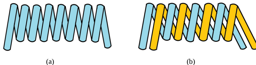
Fig. 1. Helical monofilar (a) and bifilar (b) coils.
