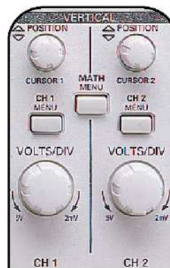
Figura 4: Controle vertical do TDS220 da Tektronix
